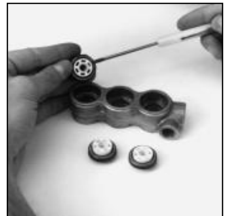
Installation of V-Packings
